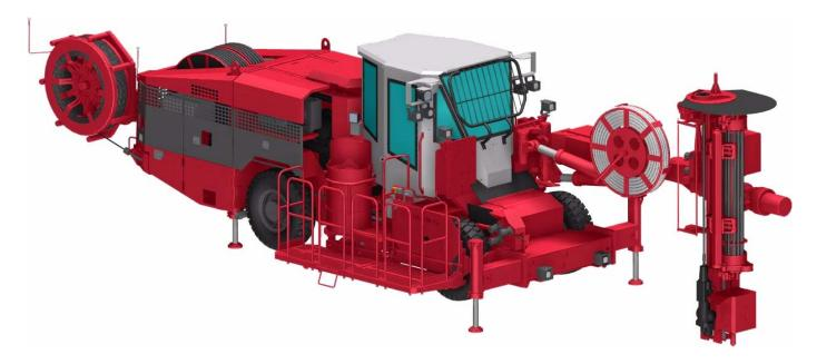
Sandvik DS421-C is a rock reinforcement drill rig specialized into cement grouted cablebolts installation in underground mines and tunnels. The Sandvik DS421-C is capable of installing up to 25 meters long cable bolts with several steel strands per hole. The drill rig is provided with an on board cement mixer, a cement bags platform and a steel strand reel. It is therefore autonomous for more than a shift.
